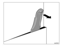
After loosening the fixing screws on the tower, push the lever between the tower and the extension piece to lever the tower out of its fixings.
